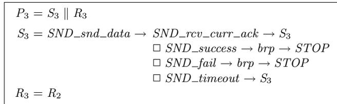
**Fig. 6.** Level 3: Control process  $P_3$
